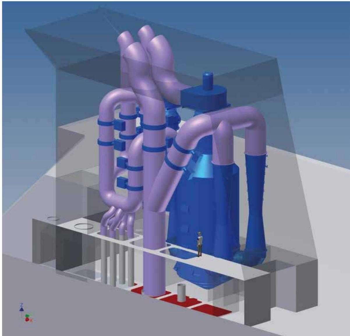
**Figure 42: Multi-stream exhaust gas cleaning unit**
