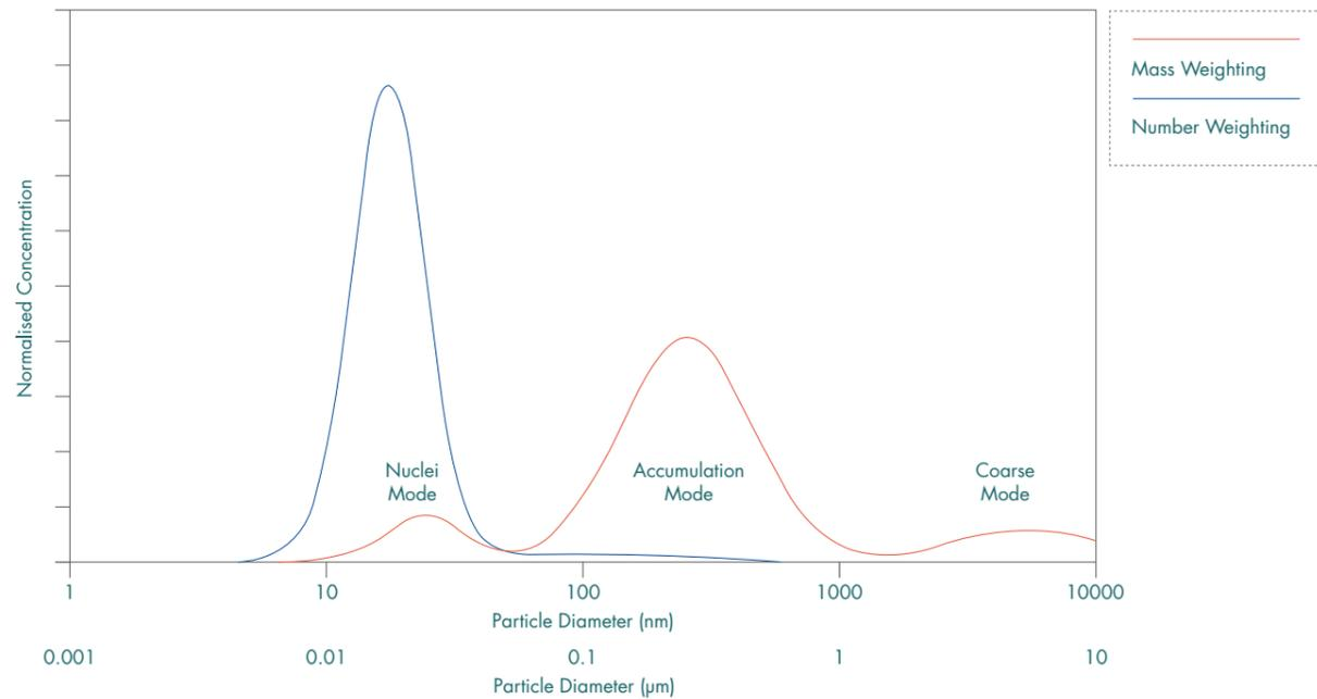
Figure 7: Graph of bimodal range of PM for diesel engines
