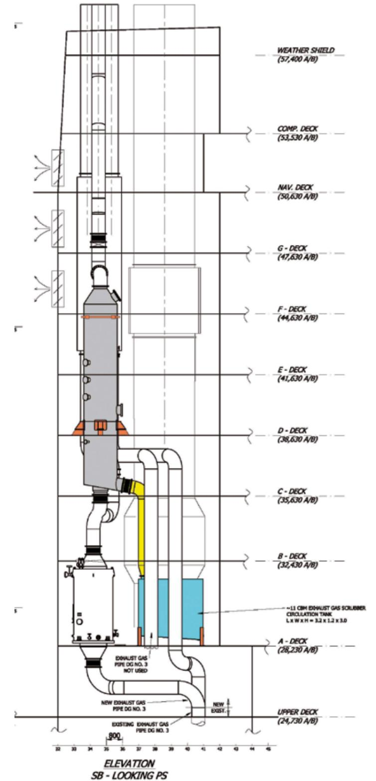
Figure 49: Exhaust gas cleaning unit arrangement – container vessel (Hybrid scrubbing system - 3.5MW auxiliary engine. Note position of circulation (process) tank is above the vessel's upper deck)
