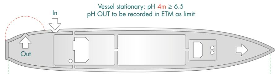
Figure 13: Measurement of position pH – Method 2
