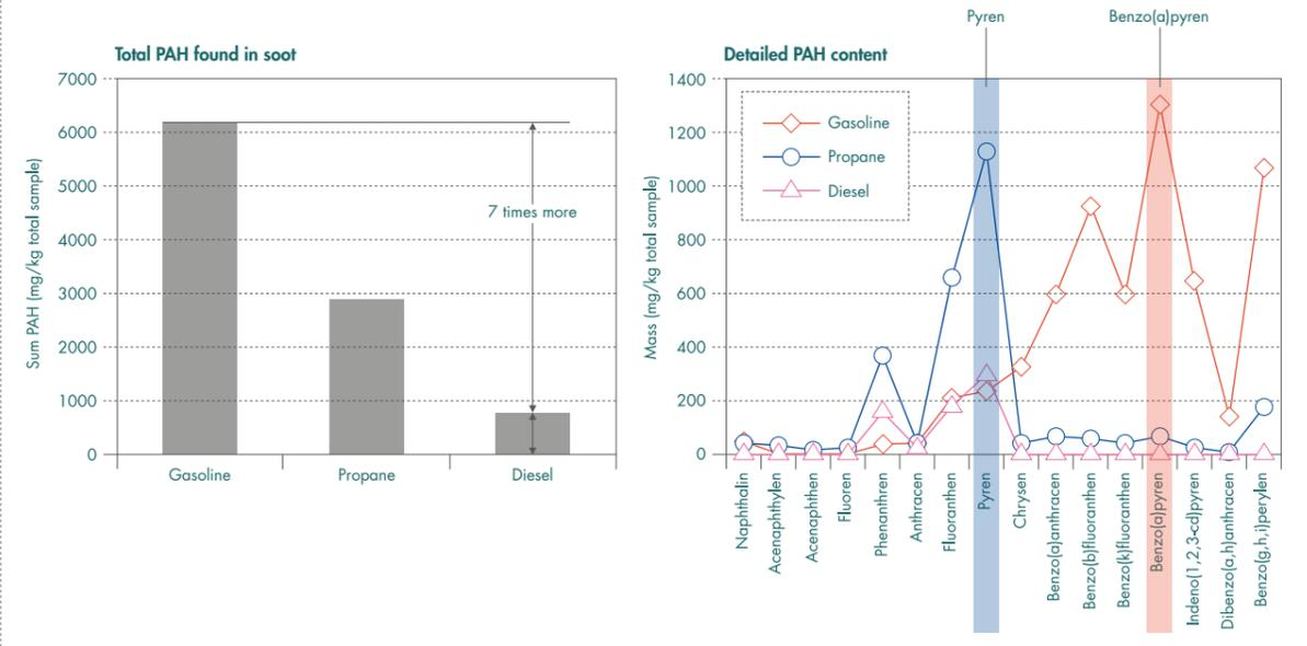
Figure 3: PAH analysis, gasoline, diesel, propane
