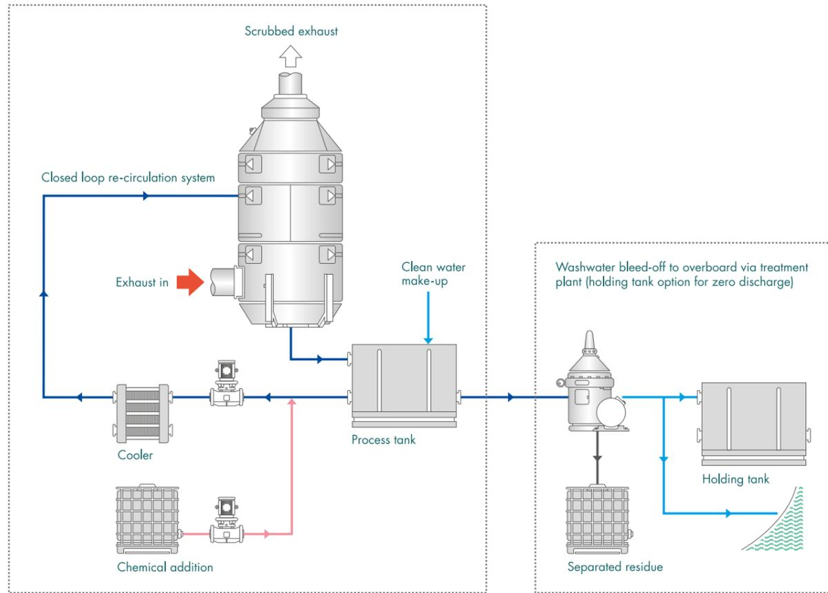
Figure 19: Closed Loop Exhaust Gas Cleaning System
