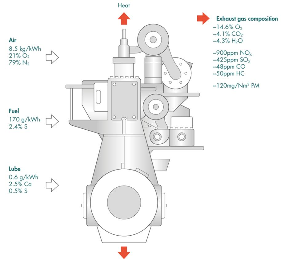
Figure 11: Typical exhaust gas composition – slow speed two stroke engine using residual fuel
