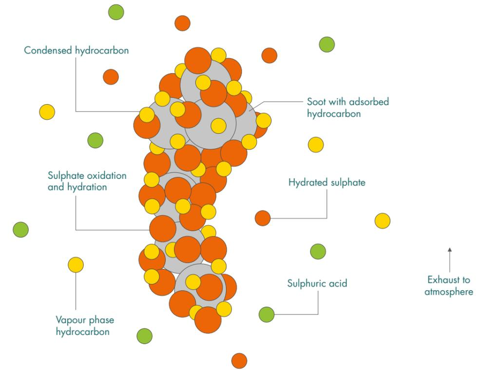
**Figure 6: Diesel engine particulate**
