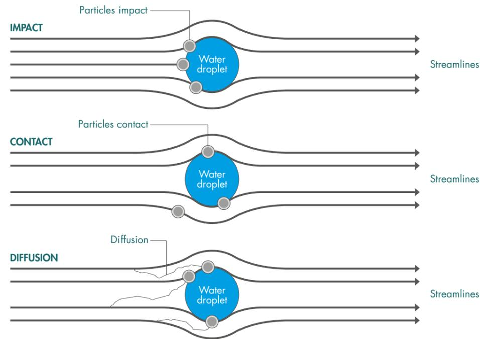
Figure 31: Particle trapping process
