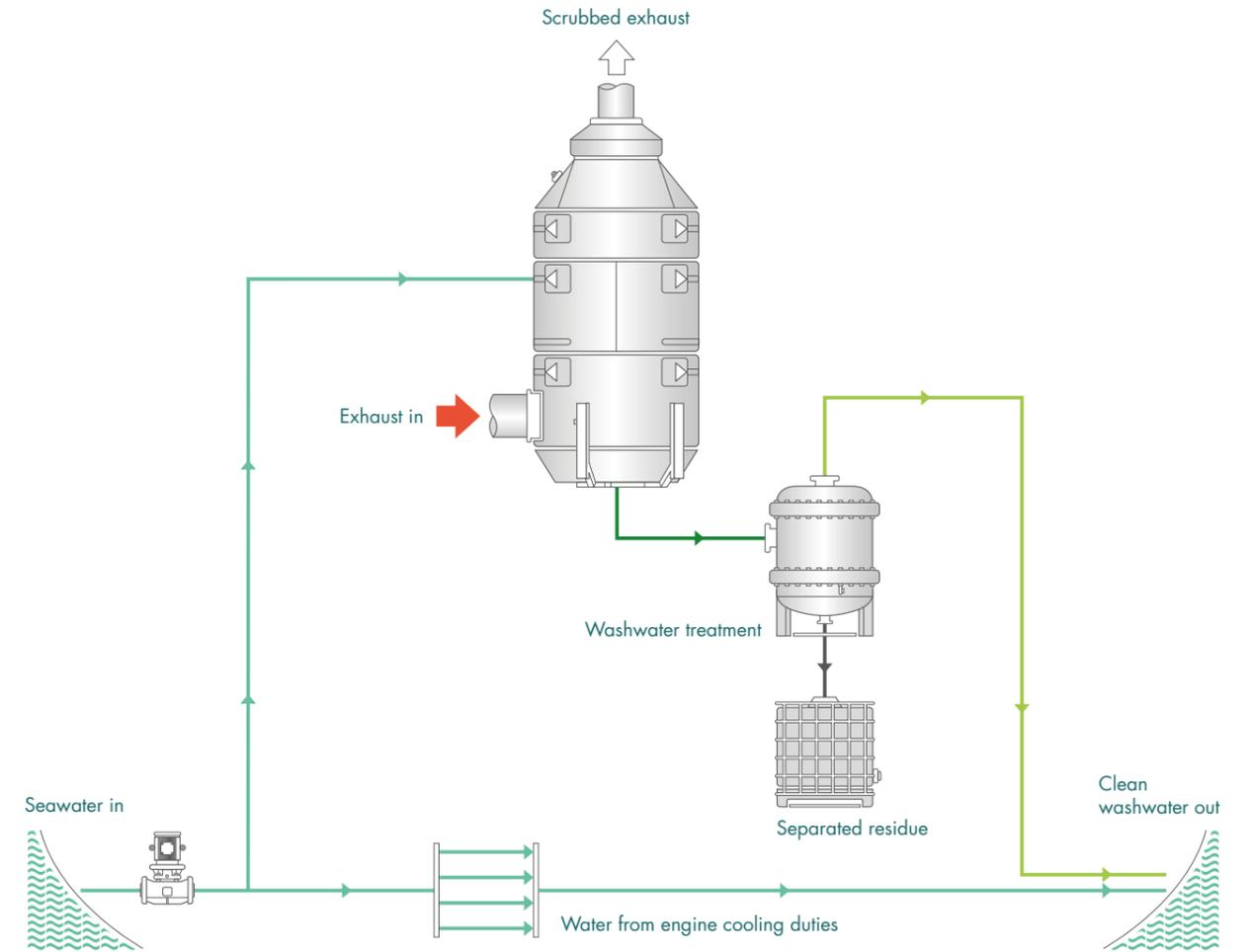
Figure 18: Open Loop Exhaust Gas Cleaning System
