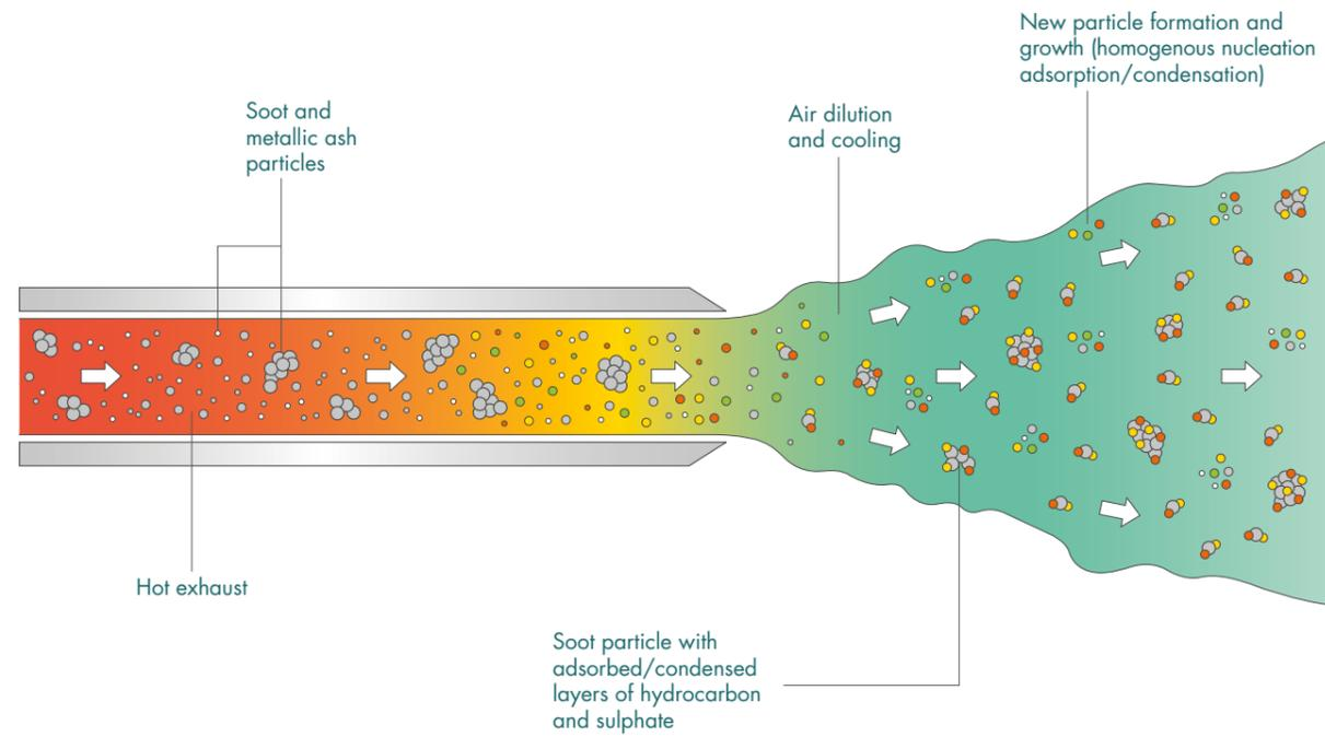
**Figure 5: The effects of cooling and air dilution**
