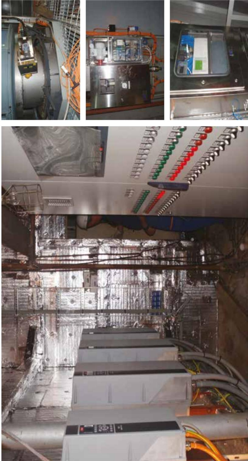
Various exhaust – actuators for bypass, insulation work new piping, top of funnel (outlet EGCS )
