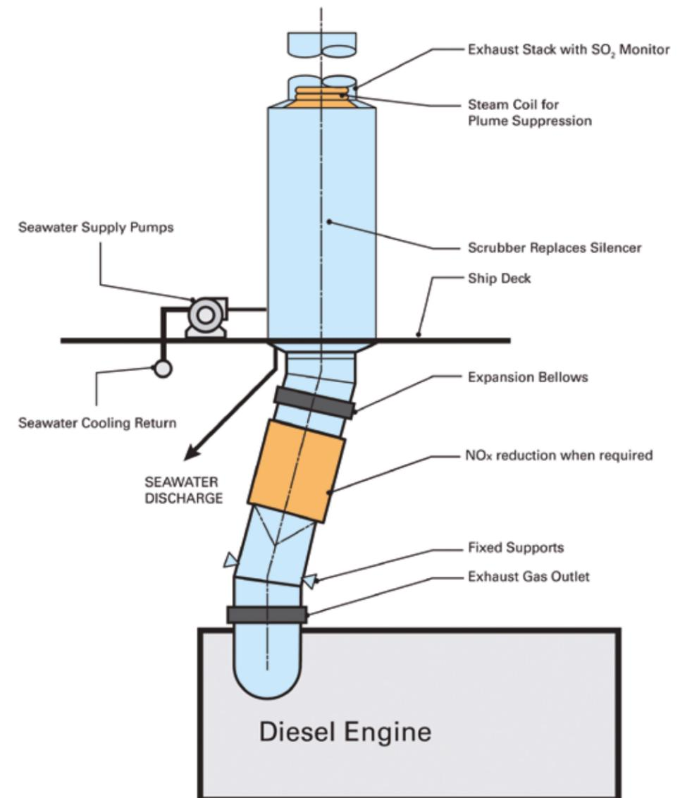
Figure 43: SCR reactor before exhaust gas cleaning unit
