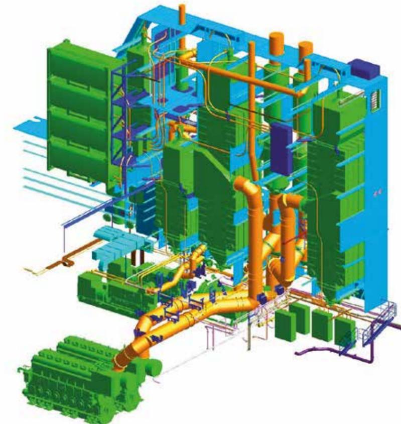
**Figure 29: Arrangement of dry exhaust gas cleaning for multiple engines**
