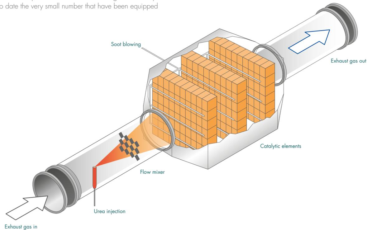
Figure 36: Selective Catalytic Reduction unit
