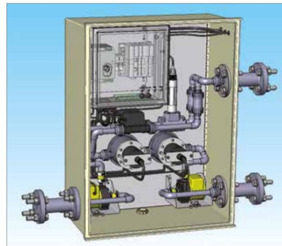
Figure 15: Washwater monitoring instrumentation cabinet (From bottom to top, left to right: sampling pumps, turbidity and PAH sensors, flow and pH sensors, control electronics)
