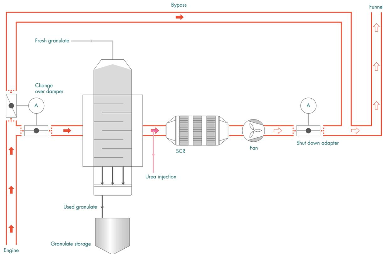
**Figure 30: Flow schematic – dry Exhaust Gas Cleaning System combined with SCR**
