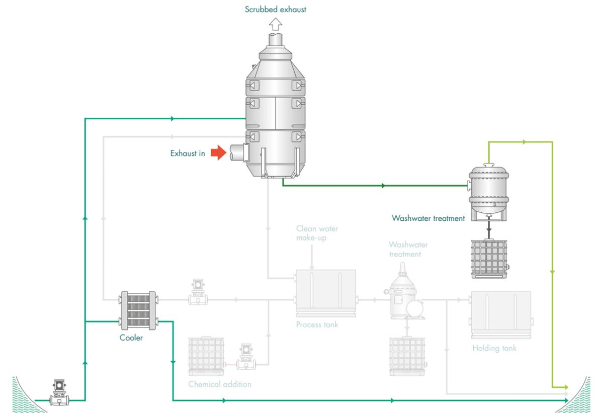
Figure 20: Hybrid Exhaust Gas Cleaning System—open loop operation
