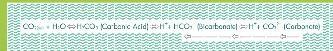
The process of exhaust gas cleaning with water creates an excess of hydrogen (H<sup>+</sup>) ions i.e. acidity of the washwater.
