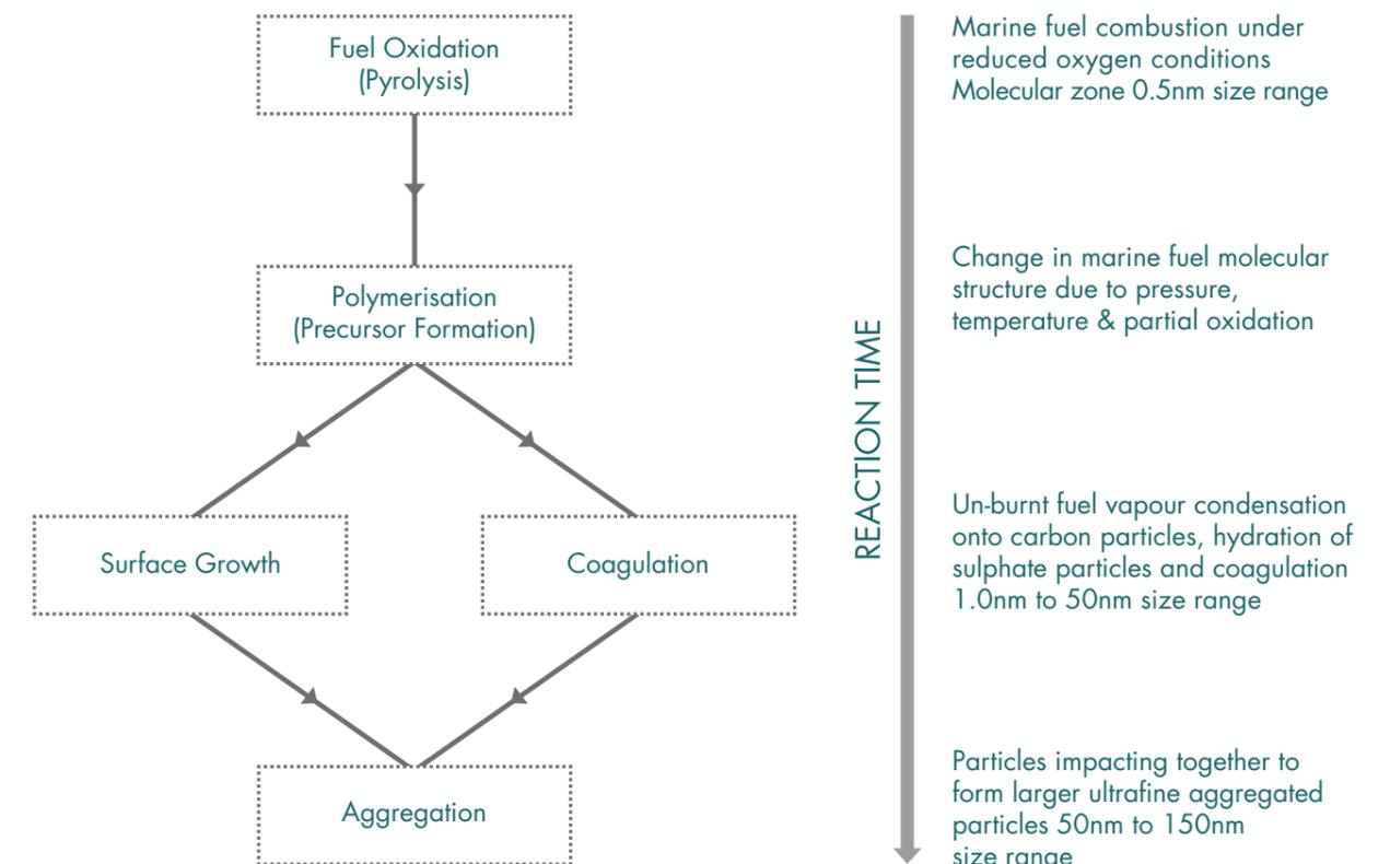
Figure 4: Particle formation – diesel engine fuel combustion
