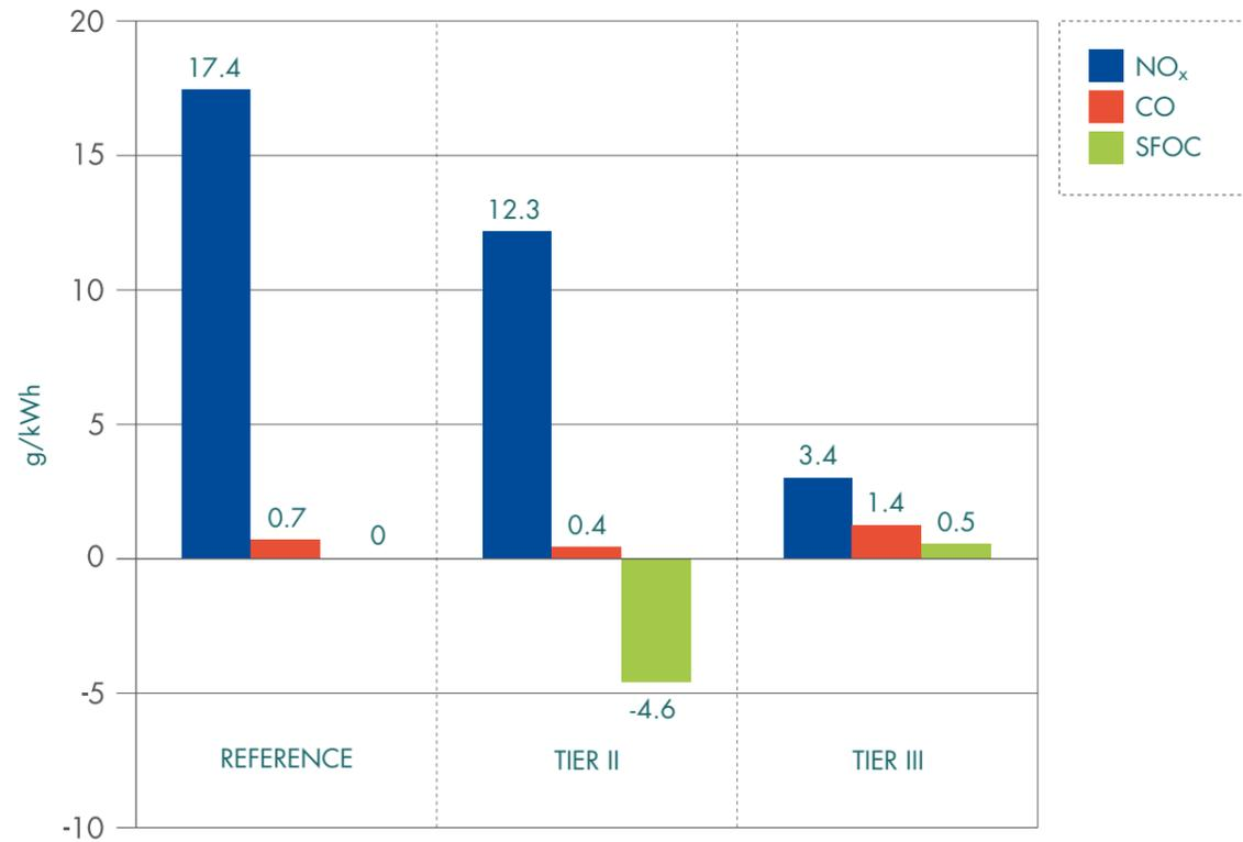
**Figure 37: Results of EGR tests on 2-stroke test engine adjusted to achieve Tier II & Tier III compliance.**
