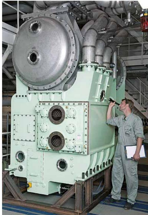
Figure 39: EGR system high-pressure scrubber unit
