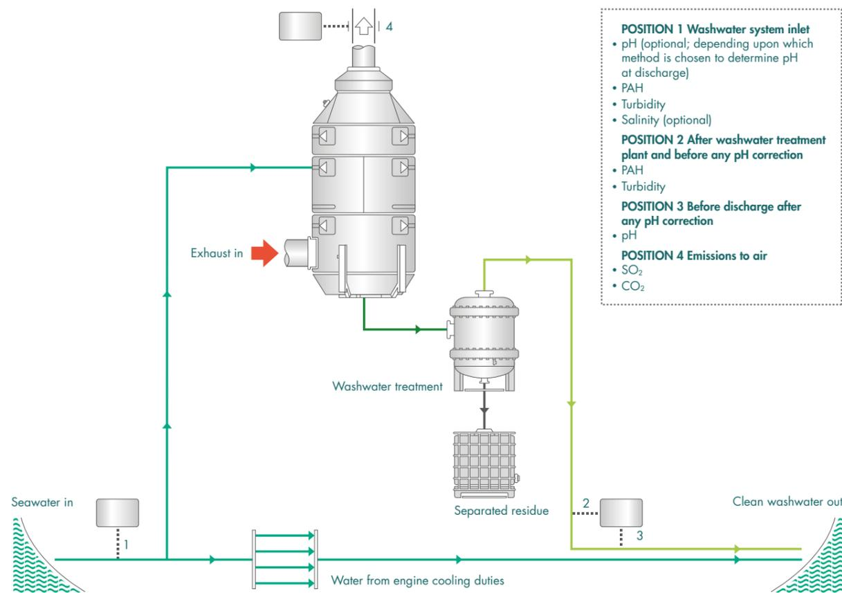
Figure 24: Position of water quality and emissions monitoring instrumentation
