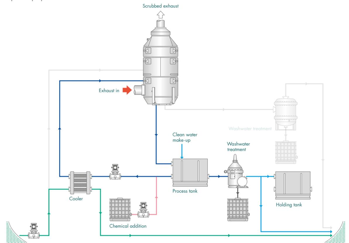
Figure 21: Hybrid Exhaust Gas Cleaning System—closed loop operation
