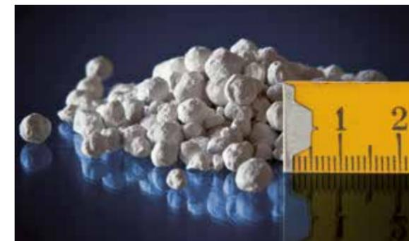
**Figure 35:** Calcium hydroxide granulate
