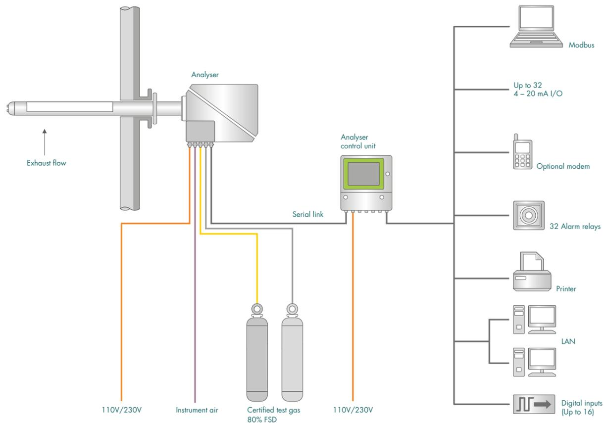
Figure 46: In-situ CEMS arrangement
