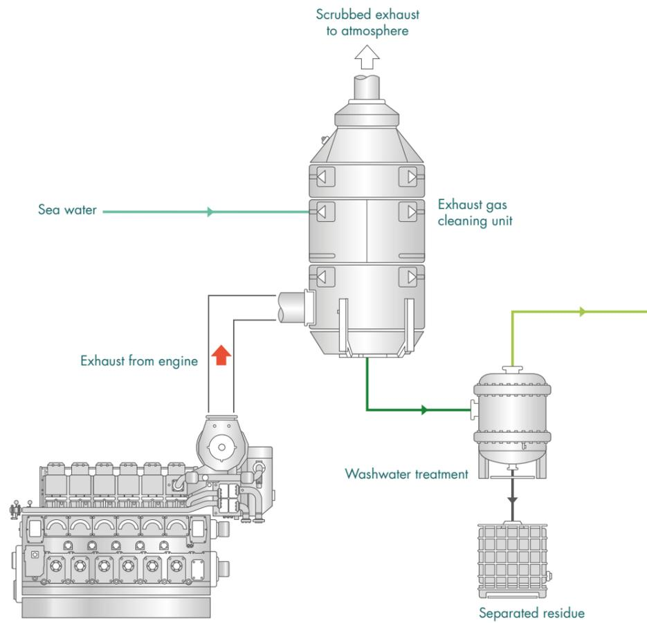
Figure 17: Exhaust Gas Cleaning System basic components
