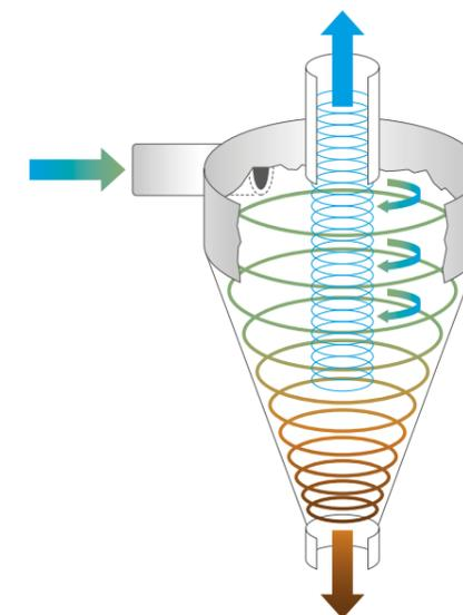
Figure 25: Hydrocyclone schematic
